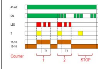
Example 1: Function E, Preset counter = 2.
