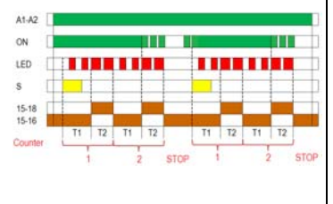
Example 2: Function Cc, Preset counter = 2.
